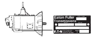
**WARNING:** Do not remove or destroy the transmission identification tag.
