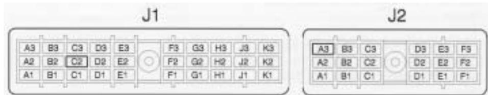
Clutch Switch Sub-Assembly Electrical
